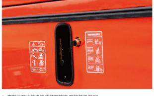
■ 高防尘防水等级电动倾翻按钮:防护等级IP67 Electric tilting button with high dust-proof and water-proof degree: protecting degree:IP67
