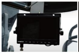
■ 后视系统(选配) 后方倒车视野可实时显示 Rear vision system (optional) truck real time rear view can be displayed when backward.
