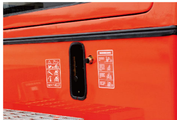
■ 高防尘防水等级电动倾翻按钮: 防护等级IP67 Electric tilting button with high dust-proof and water-proof degree: protecting degree: IP67
