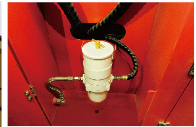
■ 进回油管用钢丝缠绕管替代胶管; 安全等级大幅提升 Steel wire wound hoses are used and safety level is improved greatly.
